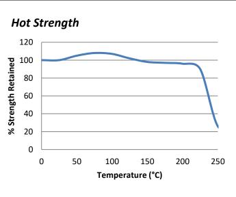
"Hot strength" shear strength tests performed on mild steel. Fully cured then conditioned to pull temperature for 30 minutes before testing. ES5504 can withstand higher temperatures for brief periods (such as for paint baking and wave soldering processes) providing the joint is not unduly stressed. The minimum temperature the cured adhesive can be exposed to is -40°C (-40°F) depending on the materials being bonded.
