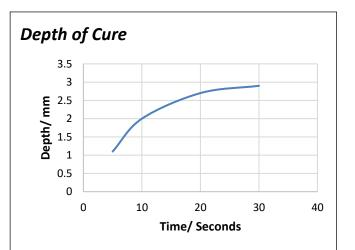
Graph shows the depth of cure at 25 mW/cm<sup>2</sup> and 405nm. The depth of cure will depend on the power of the UV lamp, its spectral output, the distance between the lamp and the adhesive.
