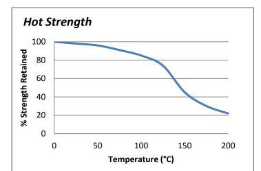
then conditioned to pull temperature for 30 minutes before testing. ES569 can withstand higher temperatures for brief periods (such as for paint baking and wave soldering processes) providing the joint is not unduly stressed. The minimum temperature the cured adhesive can be exposed to is -40°C (-40°F) depending on the materials being bonded.
