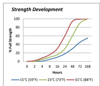
Graph shows typical strength development of bonded components. An increase of 8°C (46°F) in temperature will halve the cure time. Lower temperatures will result in a slower cure time.
