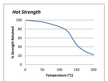
"Hot strength" shear strength tests performed on mild steel. Fully cured then conditioned to pull temperature for 30 minutes before testing. ES5748 can withstand higher temperatures for brief periods (such as for paint baking and wave soldering processes) providing the joint is not unduly stressed. The minimum temperature the cured adhesive can be exposed to is -40°C (-40°F) depending on the materials being bonded.
