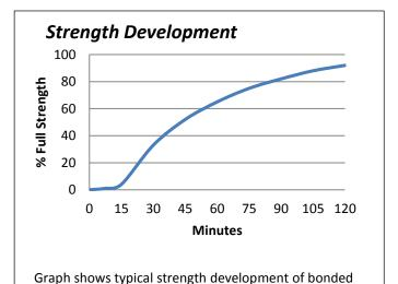
components at 23°C. Curing at higher or lower
