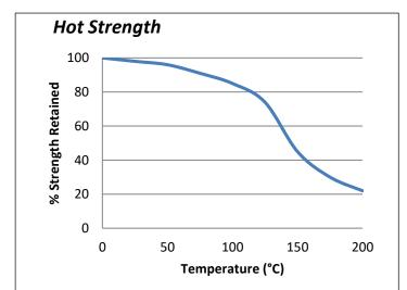
"Hot strength" shear strength tests performed on mild steel. Fully cured then conditioned to pull temperature for 30 minutes before testing.
