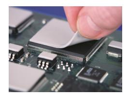
Thermally Conductive Pads - Sil Pad
