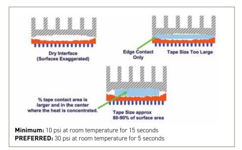
Note that typically 70% of the ultimate adhesive bond strength is achieved with initial application, and 80-90% is reached within 15 minutes. Ultimate adhesive strength is achieved within 36 hours; however the next manufacturing step can typically occur immediately following the initial application.
