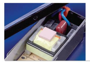
It is highly recommended that the PEN film be left intact. However, film removal will not have a significant impact on thermal performance.
