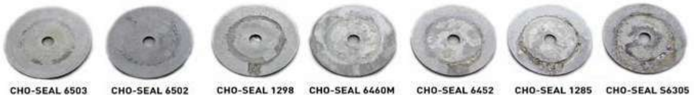
Figure 2-2 Picture of Corrosion Coupon After 504 hours salt spray / salt fog
